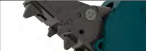
Tooth bolting style for quick and effective replacement (welding type is also available)
